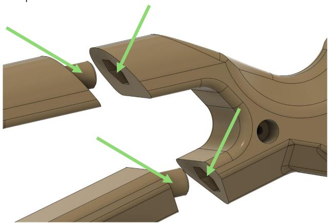
Once the stock is epoxied together, it cannot be undone without breaking the printed parts, so use some caution here and go slowly. The fit between the lugs and the hexagonal cutouts should be almost perfect with next to no play. If your parts do not fit together without resistance you will need to do some hand fitment, or tune your printer.
