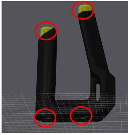
4.) Change the infill settings on the Skeletonized Stock.stl and the Modifier.stl so that the solid object Skeletonized Stock.stl has an infill of  $\sim$ 35% triangles and the modifier has an infill of 99% rectilinear.
