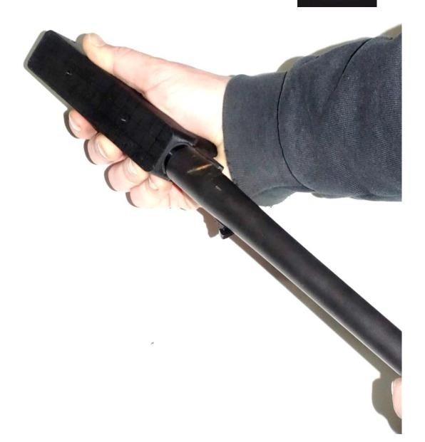
With the barrel installed all the way (it will be sticking into the inside of the receiver just slightly), spin the receiver so that the top of the receiver lines up with the top of the barrel (if your barrel has a front sight post, have the front sight post sticking up straight relative to the flat top of the receiver).
