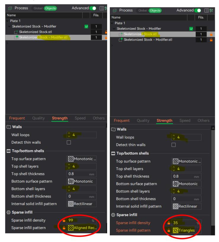
5.) Slice the file. If you used the modifiers correctly, you will notice that the lugs are solid infill and the rest of the stock is 35% triangles as pictured below.
