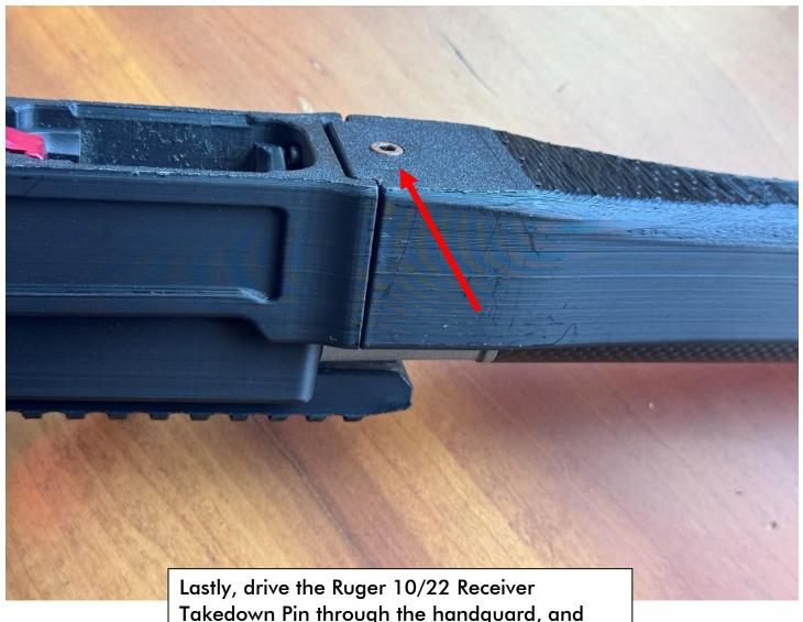
Lastly, drive the Ruger 10/22 Receiver Takedown Pin through the handguard, and into the V-Block/Retaining block, and relish in the fact that you have just created an unserialized ghost gun.
