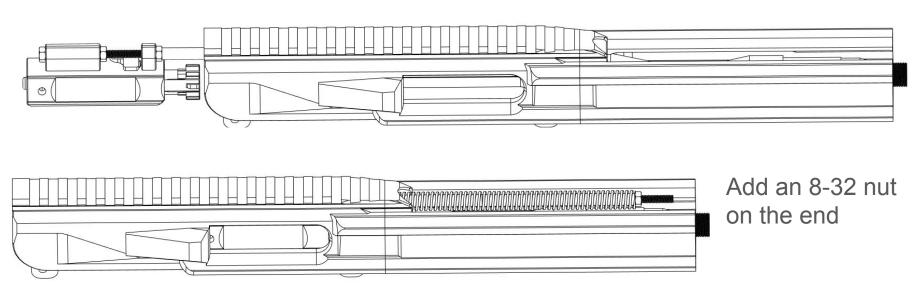
Optional: Install a G19 or G17 recoil spring to improve the pump-feel. Depending on the length you may want to shorten the spring (reduce tension) or add a portion of another spring (increase tension). A cut end should face the receiver.
