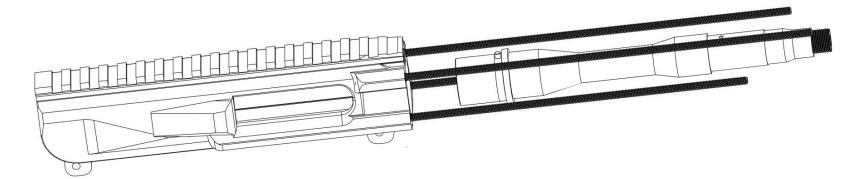
Tighten handguard down with 8-32 x ½" Binding Barrels.
