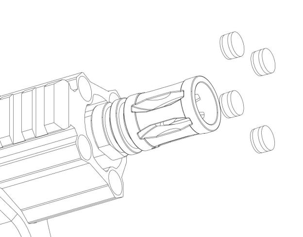
The handguard plugs can be used to hide the hardware on the front and are strictly aesthetic.
