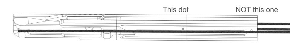
Assemble as shown, using loctite on the 8-32 nuts.
