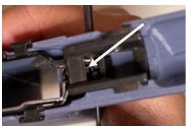
Use a punch to keep the trigger return spring taut forward to be captured by the trigger pin.
