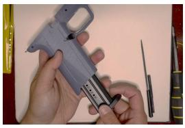
Insert a magazine and see if it fits and locks. Use the magazine release button to remove it.
