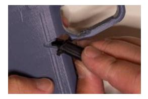
Remove debris from the magazine release geometry and test the fitment of the magazine release.
