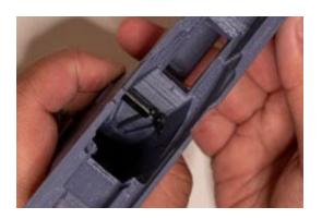
Use a flathead screw-driver to move the spring into the button.
