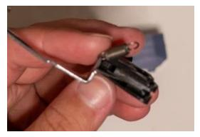
Attach the trigger return spring to the trigger bar.
