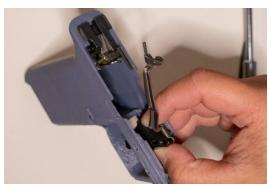
Insert the trigger into the frame, with the shoe first.
