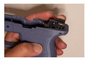
Insert the rear rail module into the frame partway.
