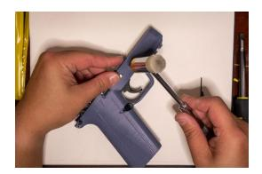
Use a frame pin to secure the front rail block.
