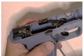
Place the slide catch on top of the trigger assembly.
