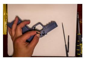
Prepare the trigger pin. Start the pin from the lefthand side of the frame.
