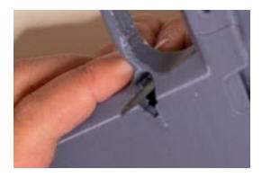
Use a stick file to clean the geometry if there is any sagging filament or debris.
