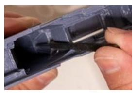
Tap on the punch gently to drive in the spring pin and secure it.
