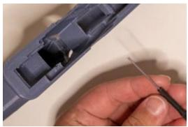
Use a 1/16<sup>th</sup> punch starter to insert the magazine release spring into the hole.
